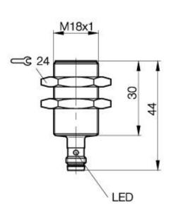
**Inductive Sensors** BES 516-326-G-E5-Y-S 49 M18x1 x 44 normally-open Sn=8mm shielded
